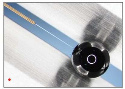
A magnified image of the target capsule that achieved ignition at the National Ignition Facility, as photographed by GA technicians after being fitting with the 2-micron fill tube. The red circle (bottom left corner) shows the actual size of the capsule.
