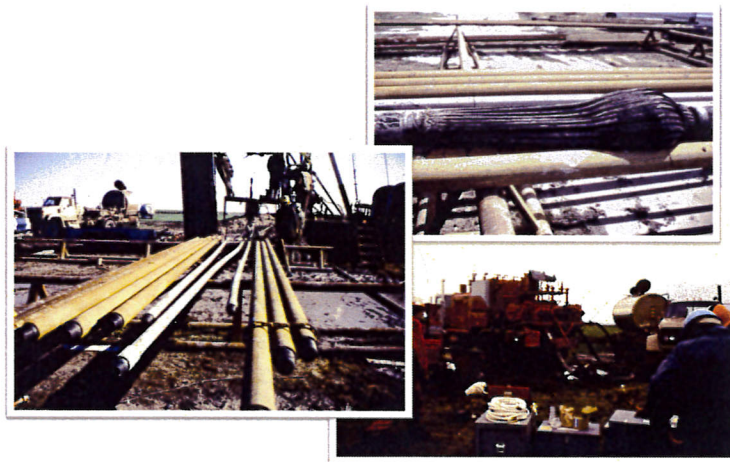
Figure 2. Regardless of the element type (inflatable for openhole or compression packer for casing), high differential pressure (pumping equipment is shown in the lower right) and temperature challenge reliability. Upper right is a failed inflatable packer. Lower left is tubing damaged as a result of energetic packer failure (refer to McLennan et al., 1986 16 ).
