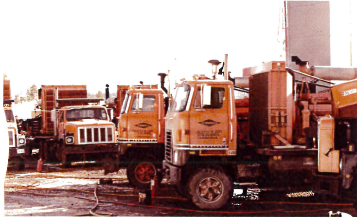
Figure 3. Part of a substantial frac fleet brought together for high rate, long term hydraulic fracturing at the Fenton Hill site in December 1983 (photograph by John McLennan).
