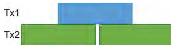
Figure H-1. A depiction of packet collisions from two transmitters (Tx1 and Tx2) showing that a single packet from one transmitter can interfere with two packets from another transmitter.
