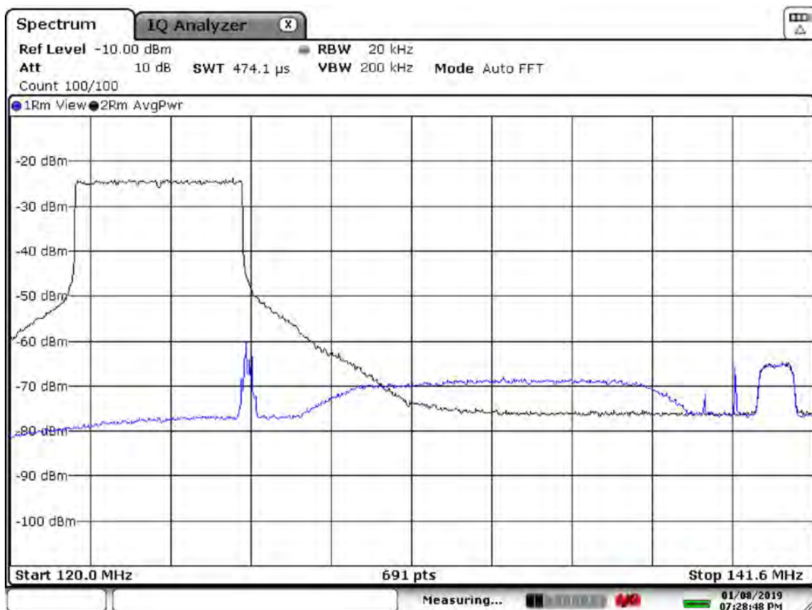
Figure 4.9-7. HRIT signal with 5 MHz LTE DL interference in 1675–1680 MHz band.
