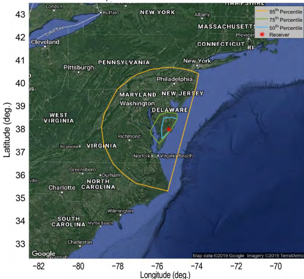
Figure 4.7-17. Composite alternate DCS exclusion zones, Wallops Island, Virginia. (Note: This map contour does not reflect the revised -128.2 dBm interference threshold from Appendix J).
