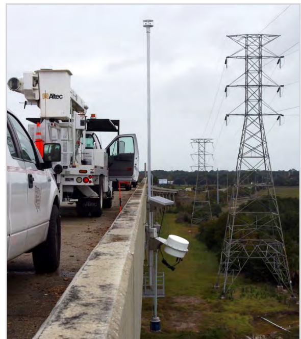
Figure 3.1-8. FDOT bridge wind speed monitors and GOES DCS antenna. Courtesy of FHWA/FDOT.
