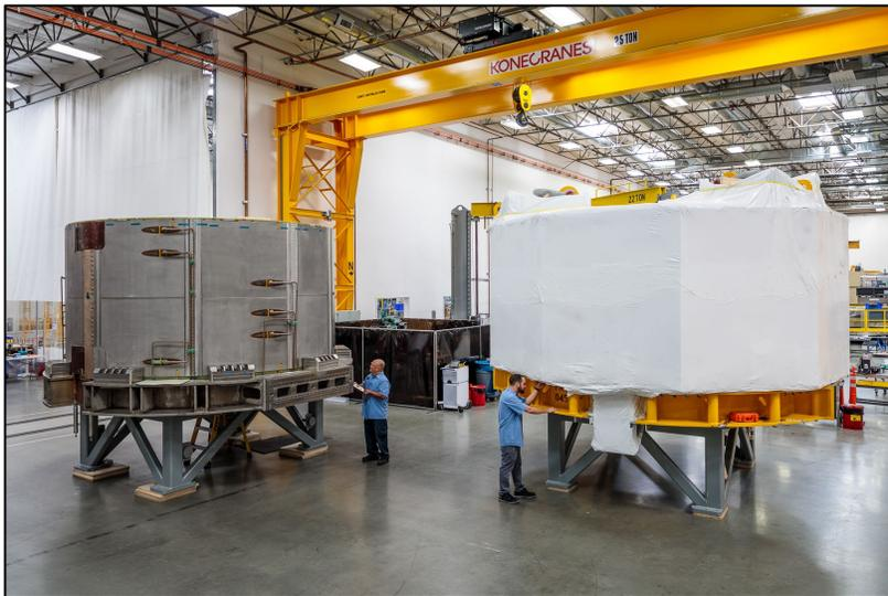
Two modules of the ITER Central Solenoid at GA's Magnet Technologies Center
