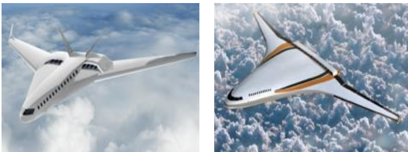
Figure 4. New aircraft concepts from the ULI (from University of Illinois Urbana-Champaign) using hydrogen fuel cells, and a NASA Turbo-Electric aircraft concept with a superconducting electric drivetrain.
