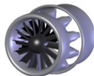
Fig. 5 New windmill design based on the engineering of jet engines
